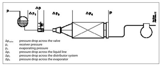
Note! The pressure drop across the liquid line and the distributor system must be calculated on the basis of the valve's max. capacity, as the valve operates with pulse-width modulation.
